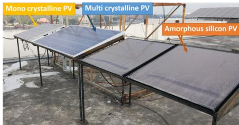
Figure 1 The installation of the three types of PV set up for the experiment.
